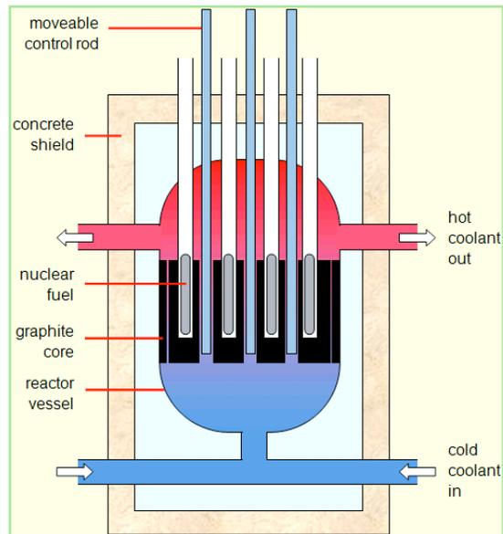
This diagram illustrates the structure of a nuclear fission reactor. The graphite core is in place to slow down the neutrons as they have to strike the fuel nuclei at a specific speed for the reaction to take place.
