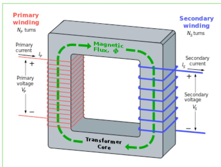
The above diagram shows a transformer. A transformer works by an alternating voltage being placed across the primary coil. This voltage will induce a voltage on the secondary coil. By changing the number of coils on either side of the core the r.m.s. value of the output current can be altered. A transformer works due to the below steps:
