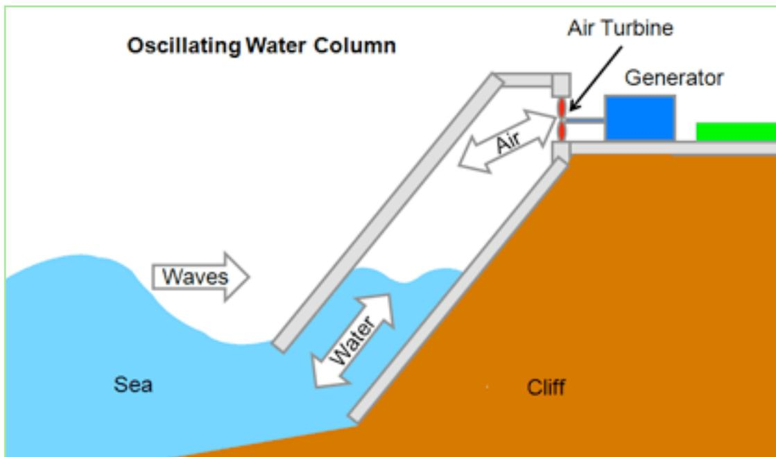
This machine works by the wave pushing water into the column compressing the air which in turn turns a turbine which generates electricity.
