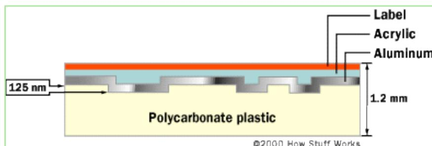
A laser is shown on the CD as it spins, when the laser is reflected off the edge of a 'bump' on the disc (each bump is the height of 1/4 of the wavelength of the light). negative interference will occur. This negative interference will be detected by the reader which will read this as a binary 1. When constructive interference occurs it will be read as binary 0.
